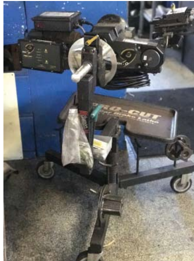
above: Custom granite top service write-up counter; EMC transmission case parts washer; Procut PFM 9.0 on car brake lathe; Snap-On D-TAC Elite battery analyzer
