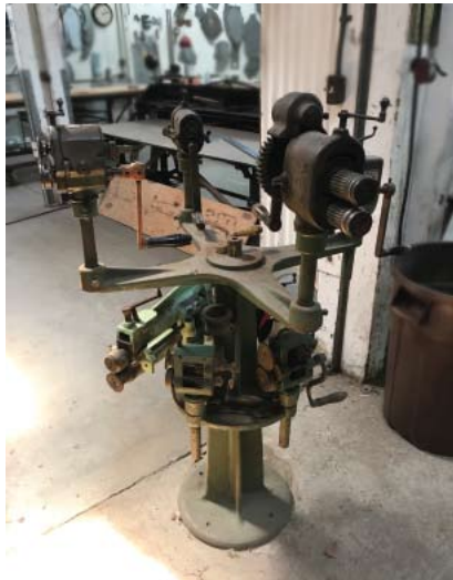
row above: Revolving pedestal metal worker with Pexto, Lockformer and Niagara shaping tools; Stryco rocker arm spot welder, model D30-15; Lockformer Pittsburgh and Acme roll former
