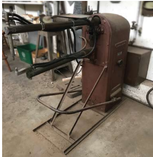
row above: Revolving pedestal metal worker with Pexto, Lockformer and Niagara shaping tools; Stryco rocker arm spot welder, model D30-15; Lockformer Pittsburgh and Acme roll former
