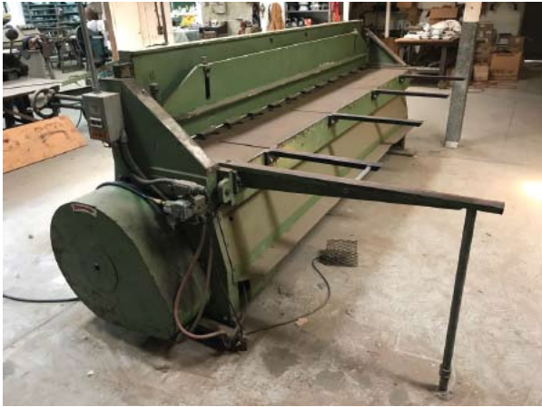
Newton 10' power shear, model 13E
