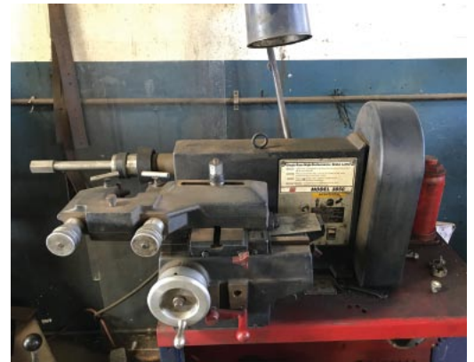
right: Ammco model 3850 brake lathe with twin facing tool
