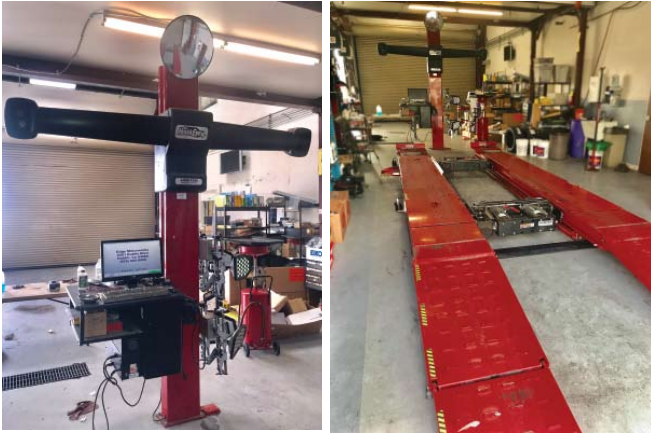
Hunter WA200 alignment analyzer with Hawkeye camera sensors and Hunter RX-12-XL scissor lift alignment rack
