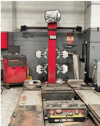
above: Rotary 9,000lb & 10,000lb win post hoists (8 total); Challenger Scissors lifts (partial view); Branick strut spring compressor; Midtronics GR8 battery station below Hunter alignment analyzer with DSP600 sensors; Hunter GSP9700 Road Force wheel balancer (1 of 2); Assorted Stanley Vidmar multi-drawer parts cabinets
